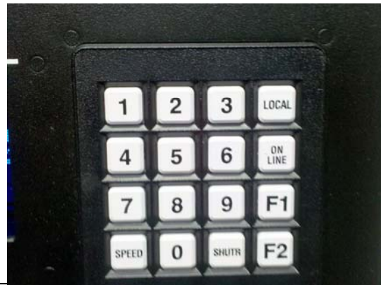
The Lambda XL Keypad will be used to manipulate the XL's LCD screen menus
