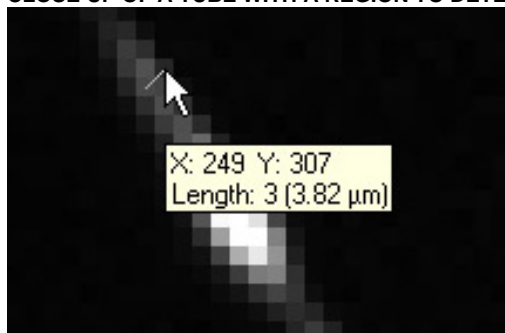
FIGURE 4 CLOSE UP OF A TUBE WITH A REGION TO DETERMINE THE WIDTH OF A TUBE
